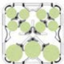
3 Columns: Dia 16.5 to 18.7cm (45 each) 8 Columns: Dia 10.8 to 11.7cm (45 each) Total Capacity: 495
