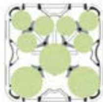
3 Columns: Dia 19.1 to 21.6cm (60 each) 6 Columns: Dia 12.1 to 13.7cm (45 each) Total Capacity: 450
